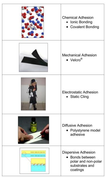
Diffusive adhesion occurs when one substrate's molecules move and intermingle (diffuse) with that of the other substrates. PVC pipe bonded with solvent-based pipe adhesive is an example of a substrate that is bonded using diffusive adhesion.
